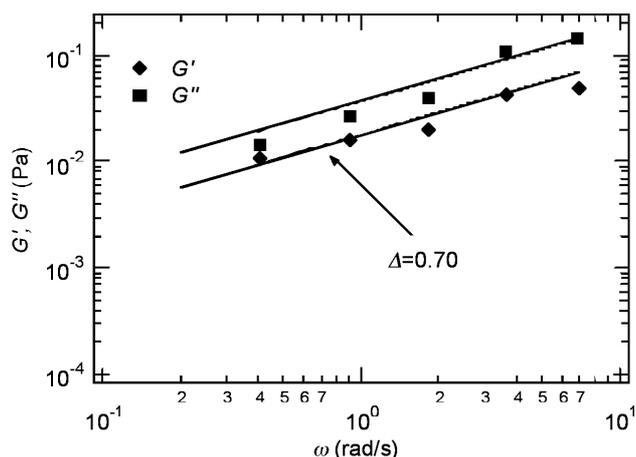
**Figure 4.** Log-log plot of the viscoelastic moduli as a function of frequency in the vicinity of the gel point at  $t = 500$  s.  $G'_t(\omega)$  and  $G''_t(\omega)$  obey identical scaling laws with an exponent  $\Delta \propto 0.70$ .
