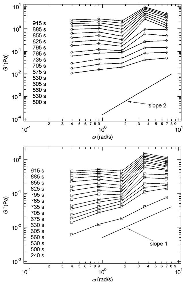
**Figure 3.** Viscoelastic impedance spectra  $G'_t(\omega)$  and  $G''_t(\omega)$  of the same collagen solution as in figure 1. The straight lines at the bottom represent the scaling laws of  $G'_t(\omega)$  and  $G''_t(\omega)$  for the Maxwell model (Fung 1993). Upper panel: storage modulus. Lower panel: loss modulus.
