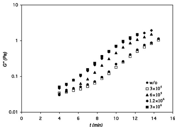
**Figure 5.** Bead concentration dependence of the viscoelastic moduli  $G'_\omega(t)$  (upper panel) and  $G''_\omega(t)$  (lower panel) ( $c = 1.7$  mg ml $^{-1}$ ,  $T = 12$  °C,  $\omega = 3.6$  rad s $^{-1}$ ). Numbers in the figures indicate the number of beads in 1 ml of the suspensions with 'w/o' denoting the bead-free solution.
